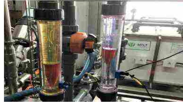
ED Plant EMU-2 for demineralization of gelatin, 24-30% TS (product quality D85). Poland, 2022
