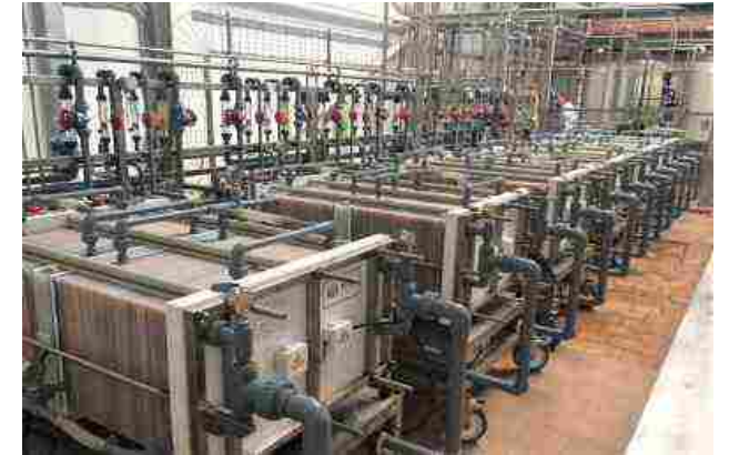
ED Plant EMU-6 for demineralization of acid and sweet whey, 24-26% TS (product quality D70). Russia, 2021-2022
