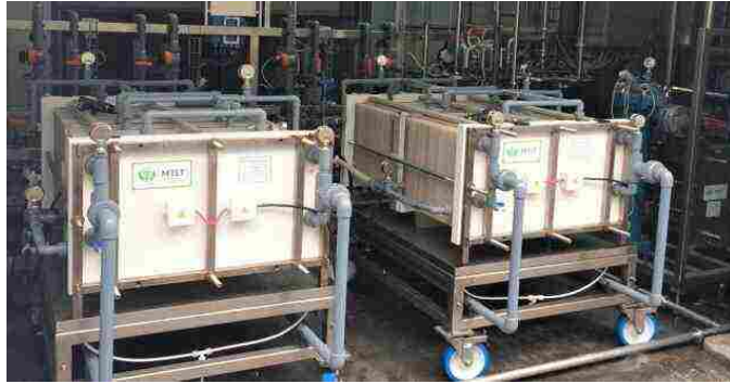
ED Plant EMU-2 for demineralization of gelatin, 24-30% TS (product quality D85). Poland, 2022
